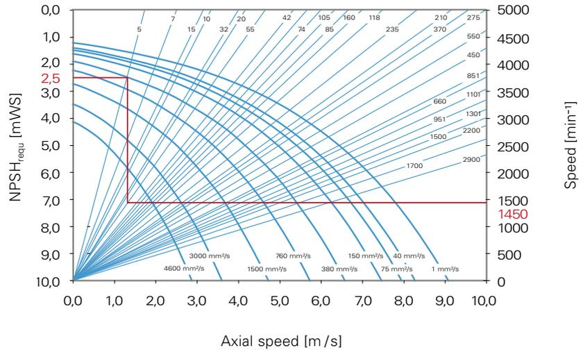
The NPSH-value (Net Positive Suction Head) indicates by how much the total pressure head at the pump inlet has to exceed the vapor pressure head  $p_d$  of the liquid to avoid cavitation. The available absolute pressure head is reduced by the suction head  $\Delta h_s$ , the pipe loss  $\Delta h_v$  and a safety margin of 2 mWS.
